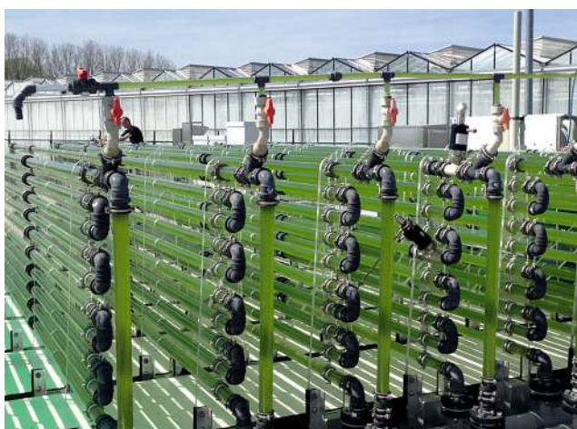
A high surface-volume ratio is one of the important design criteria for closed photobioreactors.
