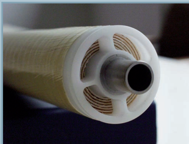
Spiral-wound modules provide an effective extension of the standard membrane module design to organic solvents.
