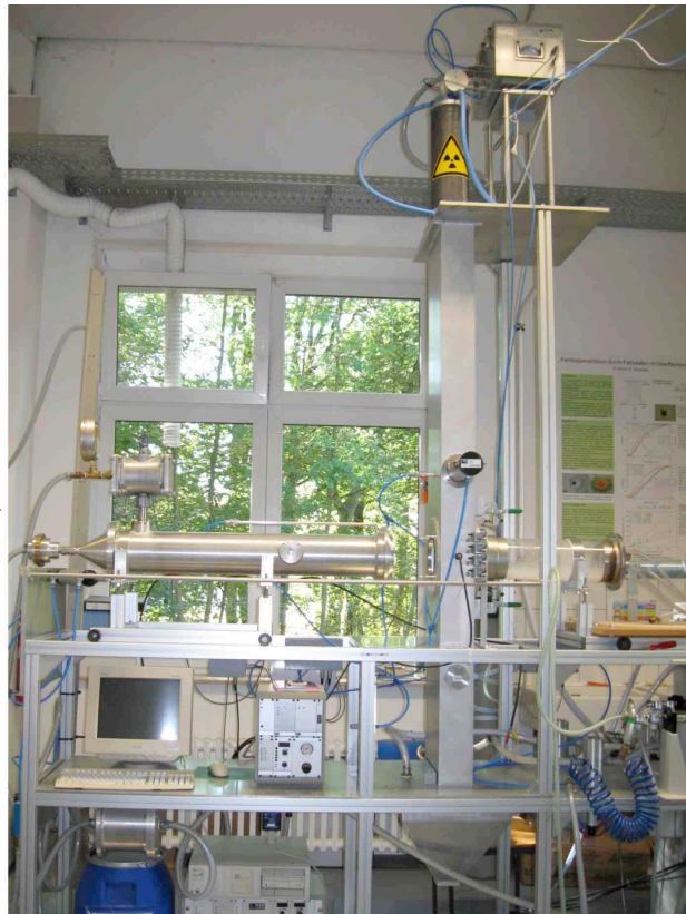
Figure 2 Scheme of a standard filter test rig according to VDI 3926-1 (l.) and photograph of the modified filter test rig used for the experimental investigations (r.).
