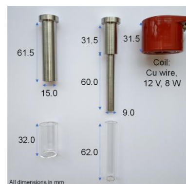
Figure 2. Electromagnet parts.
