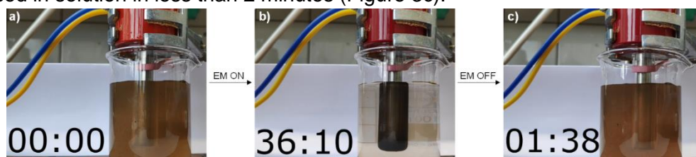
Figure 3. Reversibility of the attraction a) => b) and release b) => c) of \text{Fe}_3\text{O}_4 NPs by the EM.
