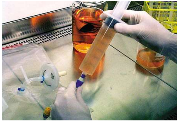
After sterile filling with culture medium and subsequent inoculation with the production organism, the desired bioreaction starts.
