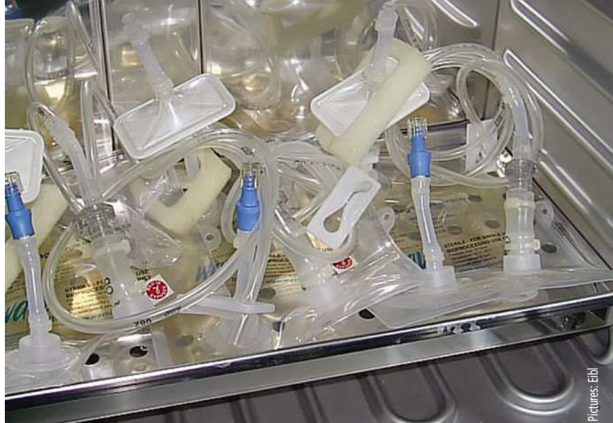
Today, disposable bioreactor applications range from cell line screening via inoculum production (picture) to glycoprotein production and, although more seldom, secondary metabolite production processes, which are most commonly realized at small- and middle-volume scale.
