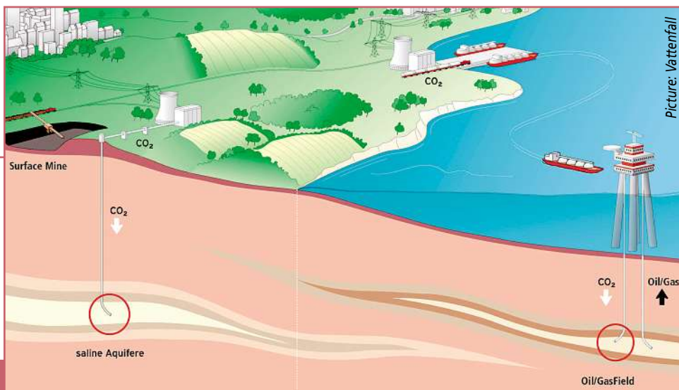
CCS technology: schematic of CO 2 storage facilities
