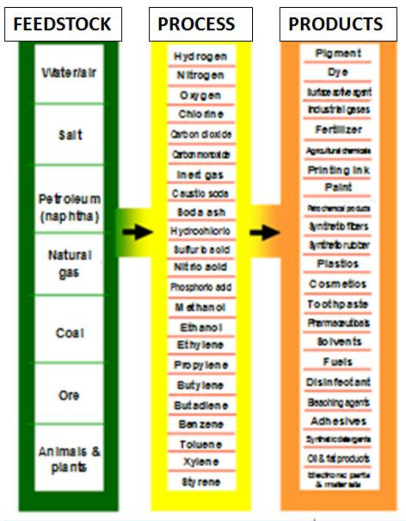
Figure 3. Illustration of chemical industry conversion of feedstocks to products.
