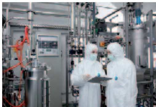
Biotech production of biological pharmaceutical actives under clean room conditions. Fermenters generate bacteria or yeasts, which are genetically engineered to secrete the desired active proteins.
