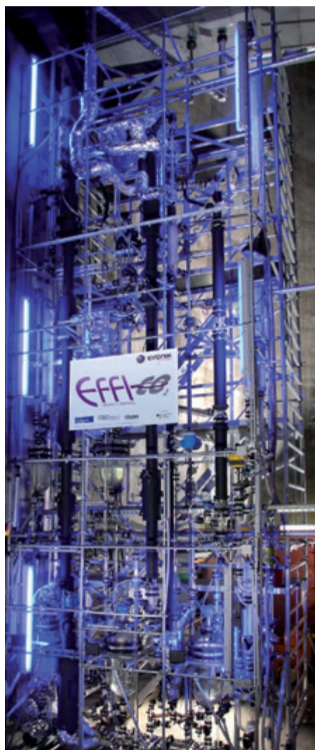
Fig. 86: The pilot carbon capture facility, which is installed at the base of the chimney in the Herne CHP plant, comprises a scrubber tower, an absorption column and a desorption column.
