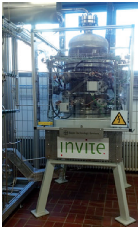
Fig. 69: Prototype of the reforming reactor
