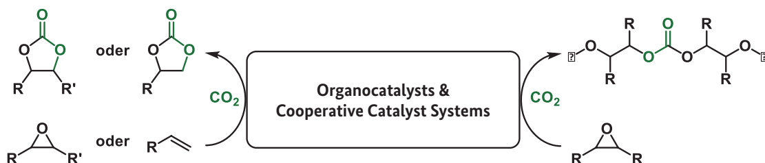
Fig. 36: Subprojects within the OrgKoKat. Left: The synthesis of cyclic carbonates from epoxides or olefins; Right: The copolymerisation of CO 2 with epoxides to form polycarbonates.
