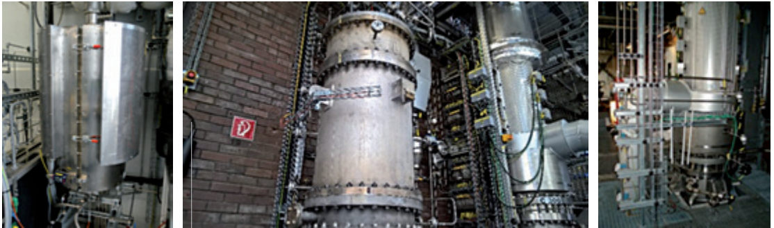
Fig. 30: Test production facilities (lab and pilot scale) for the high-temperature pyrolysis of natural gas; (2014 and 2015)
