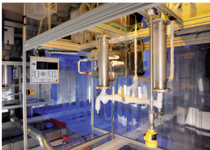
Fig. 110: Chemical heat storage test system (Source: DLR e.V.)
