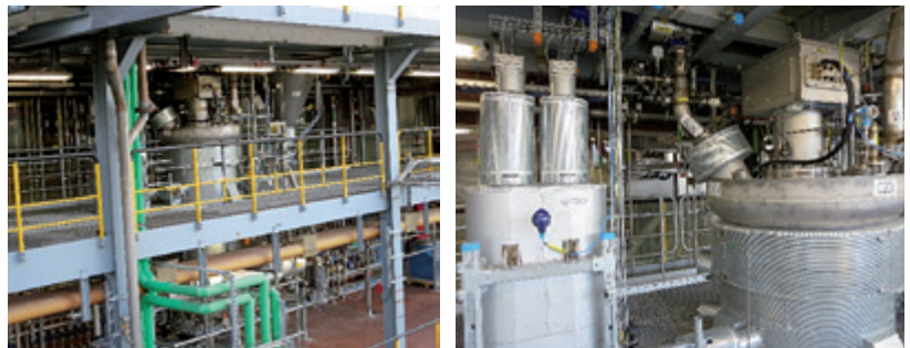
Fig. 31: Trial batch facility for the production of batches of carbon for testing; (2016)
